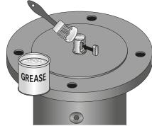
• Grease the terminal part of the gearleg shaft; fit the small key into its seat.
