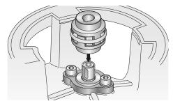
Insert the elastic joint in the terminal part of the gearleg shaft.
