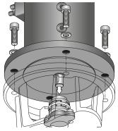
Insert the motor onto the elastic joint; fasten it with the 4 screws and washers provided.
