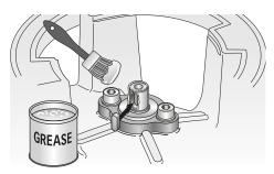
Grease the terminal part of the gearleg shaft; fit the small key into its seat.
