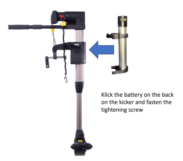
Connect the battery with the 4pin cable between the motor and the battery
