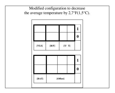
When the voltage is V<13,2(12,7) or V<25,2(24,7) DC, it is necessary to check that the average temperature is the same as the selected t value. In the standard Fridge configuration,  $t = 41^{\circ}F(5^{\circ}C)$  (to vary the t value, see Table 4.1 page 35).
