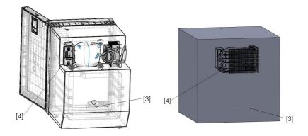
[3] 0,27in (Ø7mm) through-hole from the outside to the inside the cabinet to insert the temperature sensor.[4] Smart Energy Control circuit board
