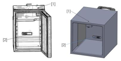
[1]  $\emptyset$ 0,5in ( $\emptyset$ 13mm) hole for installing the cable for communicating the temperature data and controlling the thermostat/electronic potentiometer temperature.
