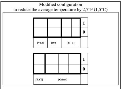
If the temperature measured is more than  $3,6^{\circ}F(2^{\circ}C)$  warmer than the <u>t</u> temperature for the selected configuration (see TABLE [1] Page 24) and the system never stops, the configuration selected is not suitable for the refrigeration system. The system has insufficient refrigerating power. Switch to a lower configuration and repeat the test e.g.
