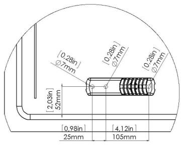
Insert the temperature sensor Fig. 1 Page 4 [6] from the outside towards the inside of the cabinet, wrap 20-27in (50-70cm) of the excess cable inside the slot formed in the covered part of the grille, and finally insert the sensor inside the small sensor holder tube, which must be inserted inside the special slot behind the grille. Close the sensor cable through-hole using the soft putty supplied in the kit or marine silicone, making sure that material does not leak into the cabinet.
