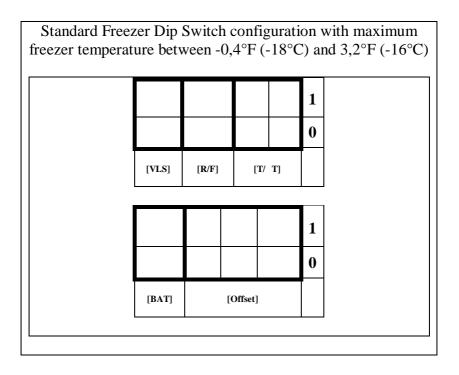
If the temperature measured is more than  $3,6^{\circ}F(2^{\circ}C)$  colder than the <u>t</u> temperature for the selected configuration (see TABLE [1] Page 24), intervene on the offset configuration, switching to the next offset, then repeat the test e.g.
