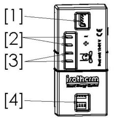
[1]: connection for the cable communicating the temperature data and controlling the potentiometer temperature.
