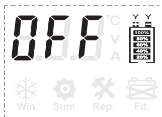
Automatically Shut Down In 2 Hours After Fully Charged
