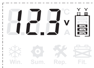
Normal Charging When Current, Voltage And Temperature Display In Rotation, And Power Level Blinks Successively
