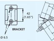
The rear bracket allows a 125° oscillation range of the actuator
