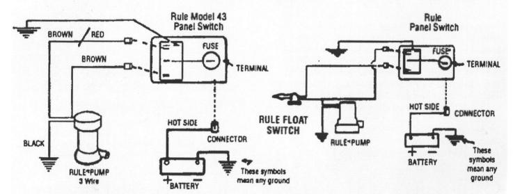
THIS PRODUCT SHOULD BE FUSED WITH THE RECOMMENDED FUSE SIZE FOR THE RULE PUMP TO WHICH IT IS CONNECTED.
