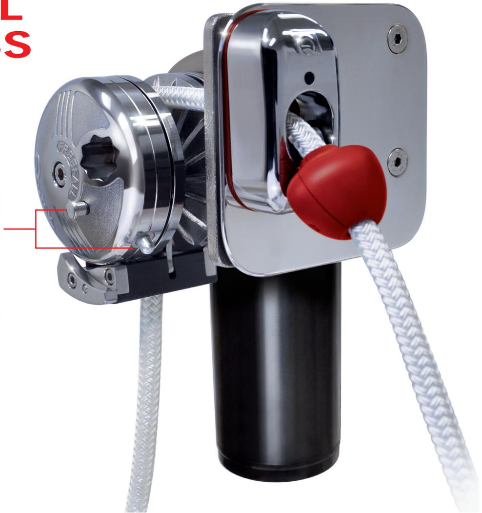
The **Automatic Free-Fall System** applied to the Balder windlass allows free running of rope through the gypsy when lowering the anchor; simply by depressing the down control button the windlass will release its clutch and the gypsy will freewheel. To stop the Free-Fall depress the up control button on the windlass; the clutch will engage stopping the gypsy and allowing retrieval of the rope. The Free-Fall function can be bypassed to facilitate power controlled release.
