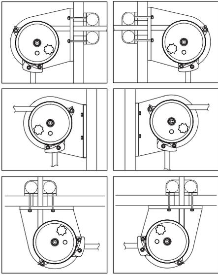
The mounting bracket allows the user to install the windlass in a variety of combinations.
