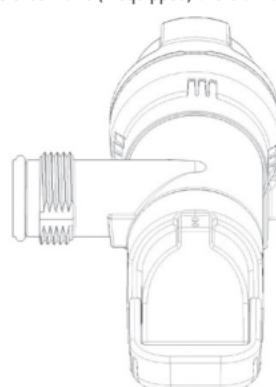
Please note that the check valve should NOT be used with the elbow fitting. The check valve and elbow combination greatly restrict the flow.
