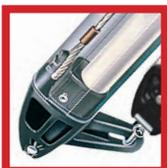
The extended block attachment lug allows the block to turn, enabling the tackle to be operated from either port or starboard. The Rodkicker is supplied with detailed instructions and is easily fitted. If a Rodkicker is retrofitted to an existing rig, the original kicking strap tackle can still be used. Seldén Rodkickers are made of anodised aluminium and are carefully tested to meet stringent quality and performance standards.
