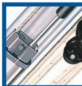
The Rodkicker can be supplied with an optional integral gas spring. This lifts the boom when the kicking strap is released, opening the leech of the sail. A Rodkicker with a gas spring replaces the topping lift, making reefing fast and simple. The gas spring is easily retrofitted to a Rodkicker that does not have a spring.
