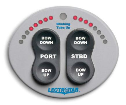
Pictured above is the SETR-50 with black switches on a gray background. The SETR-51 is identical except for the color, wherein it has black switches on a black background. The actual size is about 4" wide, 3 ½" high and ½" deep.
