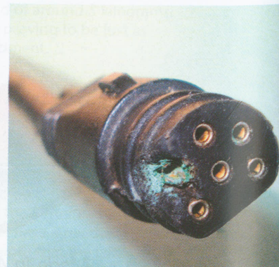
A sounder plug which has been badly corroded as a result of battery power being left connected for long periods when the boat is not being used.
