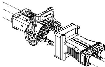
Figure 4.12 High-voltage interlock pconnector - Installation step 1
