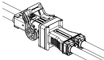
Figure 4.14 High-voltage interlock pconnector - Installation step 4
