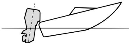
Excessive inward trim makes the boat "plow" through the water, leading to difficulty in accelerating. Running at high speeds with excessive inward trim can also make the boat unstable. The resistance at the bow significantly increases, making steering difficult and hazardous.
