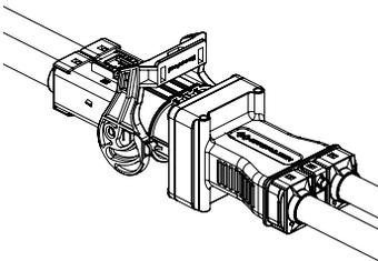
Figure 4.13 High-voltage interlock pconnector - Installation step 3
