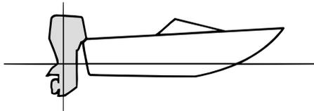
Excessive outward trim raises the bow too high in the water, causing increased resistance, reduced performance, and fuel efficiency. It can also lead to the propeller partially coming out of the water, further reducing performance, and causing the boat to "porpoise," ejecting the operator and passengers.
