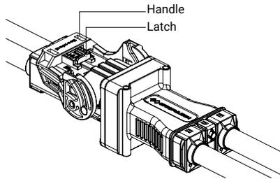
Figure 4.15 High-voltage interlock pconnector - Installation step 5
