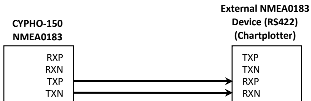
Figure 8 NMEA0183 Connection illustration
