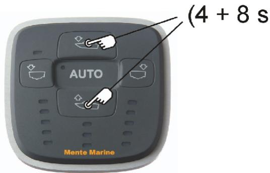
The AUTO indicator blinks to indicate that calibration is needed. Press the uppermost and lowermost buttons simultaneously for 4 s to start the calibration. Keep the buttons depressed for another 8 s while the ACS is calibrating.
