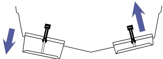
Should the trim tabs move in the wrong direction: For hydraulic trim tabs, exchange the 3 and 4 wires, for electromechanical trim tabs, exchange the 3 and 4 wires with the 5 and 6 wires.
