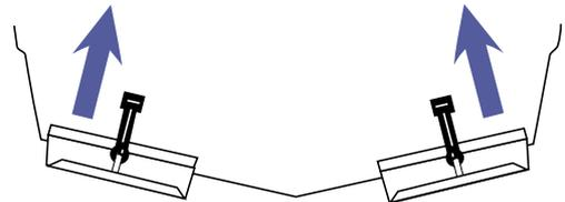
Should the trim tabs move in the wrong direction: For hydraulic trim tabs, exchange the 5 and 6 wires, for electromechanical trim tabs, reverse the wires of the actuator(s) that move in the wrong direction.
