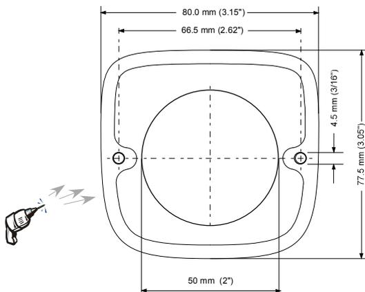
Choose a location close to the helm where the control panel is easy to access and drill holes for the screws and connectors using the enclosed drill pattern. In retrofit installations, remove the old panel and use the new panel to cover the hole.
