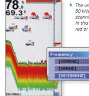
> The unit can be either set for single frequency operation, 50 kHz or 200 kHz, at your convenience, or for dual frequency scanning, as shown in this image.
