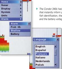
> The Condor 340c has three different alarms that instantly inform you about the fish identification, the shallow water and the battery voltage.
