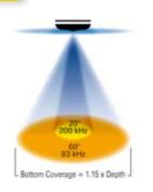
The unit can be either set for single cone operation, large 83 kHz or narrow 200 kHz, at your convenience, or for DualCone scanning, as shown in this image.
