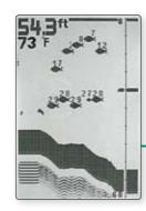
Thanks to its sophisticated identification software, the F-238 identifies any suspended target, such as fishes, showing them on the screen as fish icons, with the digital readout of the depth above them. Experienced users can anyway disable this feature at any time, getting on the screen the actual echo returns, that show on the screen important details such as thermoclines, baitfish and fish movements.
