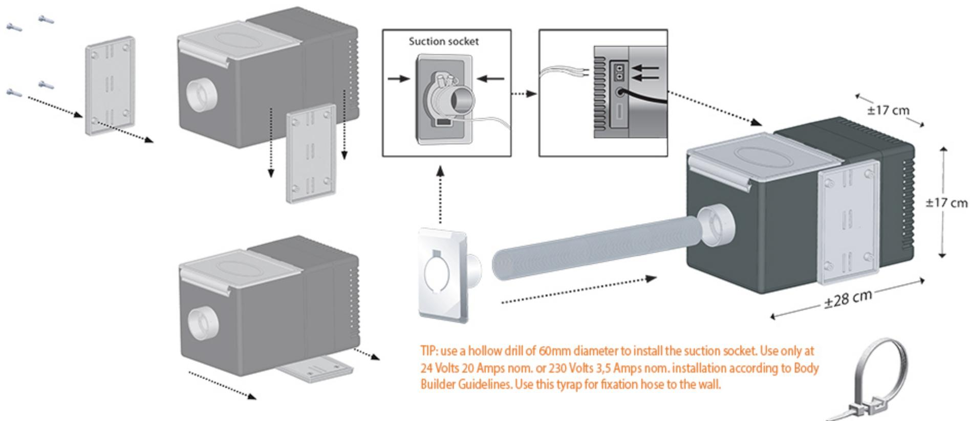
TIP: use a hollow drill of 60mm diameter to install the suction socket. Use only at 24 Volts 20 Amps nom. or 230 Volts 3,5 Amps nom. installation according to Body Builder Guidelines. Use this tyrap for fixation hose to the wall.
