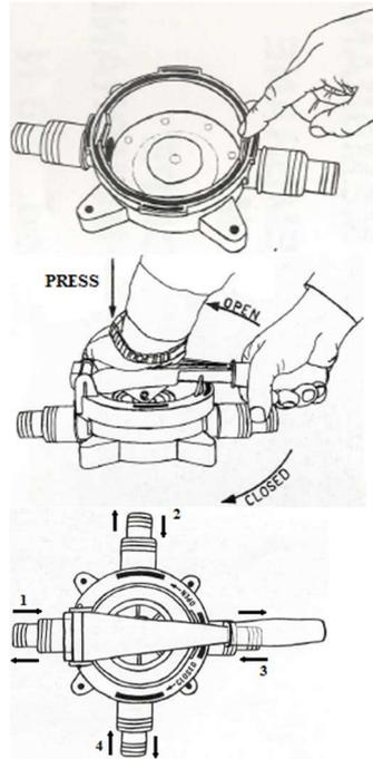
It is advisable to oil the upper rim of the pump before replacing the membrane.
