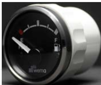
Fuel 12V/24V 110620 / 110625 0 - 190 / 240 - 30 Ω Ø54 MM
