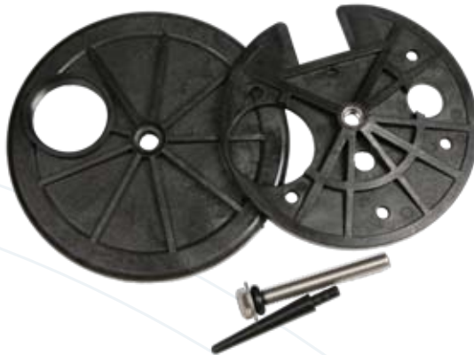
FLB-1 163110 (closed) - 163120 Inspection flange, nylon, manhole. One hole 1 1/4" BSP for S3/S3H sensor. Tankhole: 115 mm Outer diam: 150 mm
