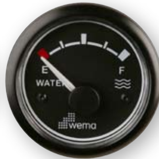
WATER 110310 - 110315 12V/24V 0-190 \Omega - 240-30 \Omega Ø54 MM
