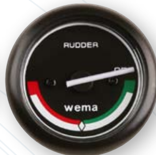
RUDDER INDICATOR 110080 12V/24V 0-180 \Omega Ø54 MM
