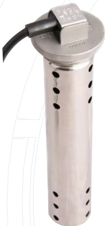
S3H Holding tank Stainless steel 1 1/4" BSP 100-760 mm 12V/24V 240-30 \Omega
