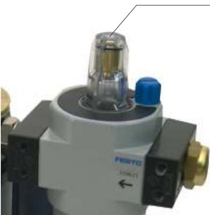
The lubrication is regulated by means of this small screw. Unscrewing the brass screw, using a screwdriver increases the oil flow and consequently the lubrication of the membranes. While screwing the brass screw, decreases the oil flow and therefore the lubrication of the membranes is reduced. For the first time filling use the oil supplied in the kit. For future refilling use lubricator specific oils or, alternately, ISO VS32 type oil or SAE 30 automotive oil.
