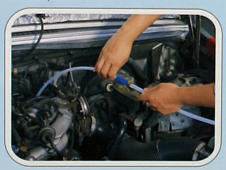
5. When the fluid inside the extractor tank reaches "Full" position, the Extractor Unit will shut off automatically, the Handle ( H ) of the Hand Pump ( G ) will lock. Push the Release Button ( B ) on the side of the Cover Housing (A ), then press the Handle ( H )of the Hand Pump ( G ) to the bottom position to release Hand Pump from the locked position.
