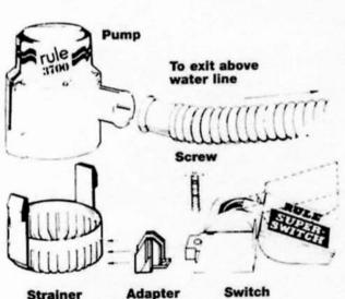
**STEP 2** Determine the desired location for the pump. If only one pump is used it is usually where the water is deepest in the bilge while the boat is at rest. The installation must allow for complete drainage of the hose. All water pockets must be eliminated by having the hose running level or continuously upward.
