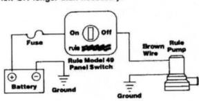
Wiring for Automatic Operation
