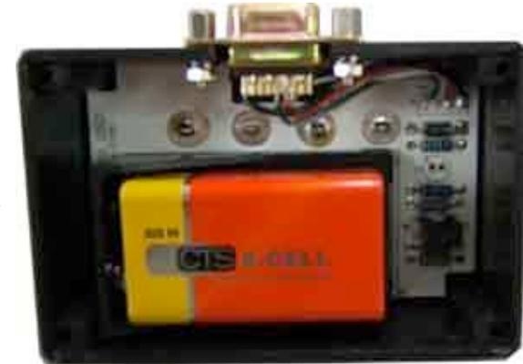
TS1-PK with 9V Battery installed
